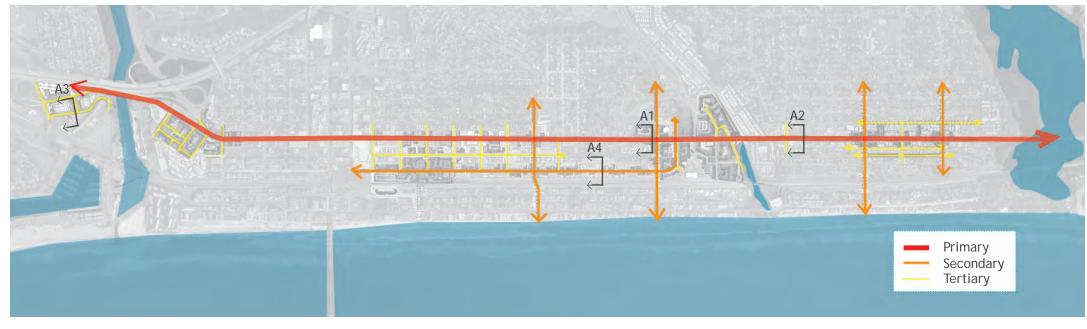
The diagram shows the hierarchy of street standards within the Planning Area. Coast Highway - in red - is the primary thoroughfare for this area - with greater street width, higher speeds, and heavier traffic flows. The streets outlined in orange are considered secondary streets - of smaller size and width with less traffic flow and lower speeds. The last set of streets, highlighted in yellow, are tertiary streets. Street sections for A1-A4 are illustrated on the facing page.
