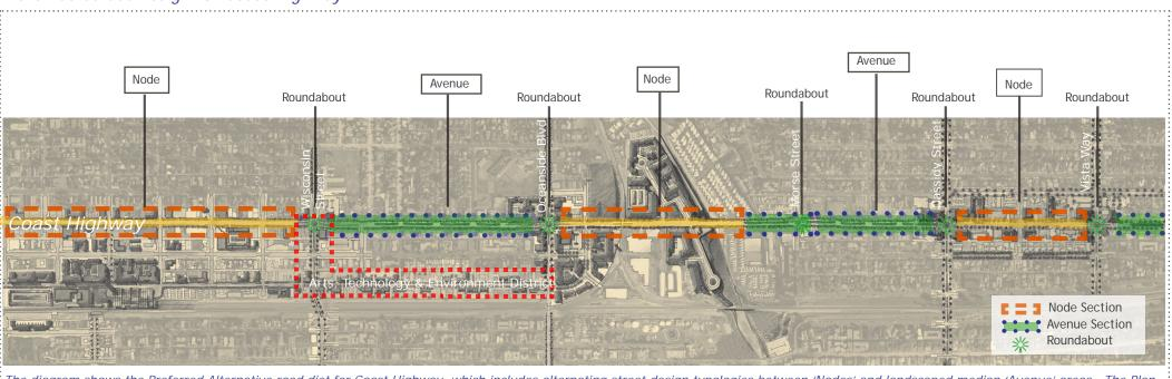
The diagram shows the Preferred Alternative road diet for Coast Highway, which includes alternating street design typologies between 'Nodes' and landscaped median 'Avenue' areas. The Plan
