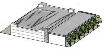
Parking garage placed behind street-facing retail buildings. Structured parking maximizes land used for parking by building "up", rather that "out." It is less expensive than underground parking and easier to share, as in a "park-once" garage. However, the garage should be screened or hidden from primary streets.
