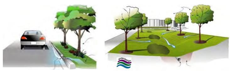
Sustainable stormwater design, directing runoff into vegetated parkway to absorb and filter water.
